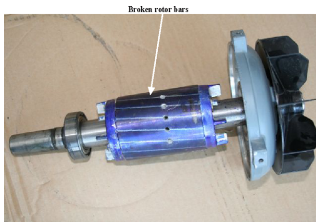
Fig. 2. Broken rotor bars.
